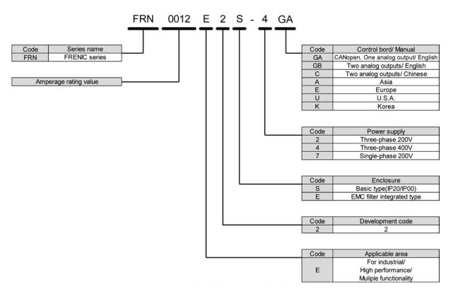
Figure 1.1-2 Type of inverter
