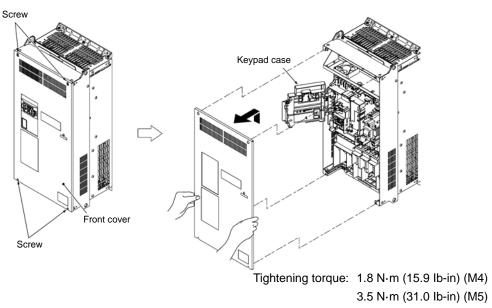
Figure 2.2-6 Removal of the front cover (for FRN0203E2■-4□)
