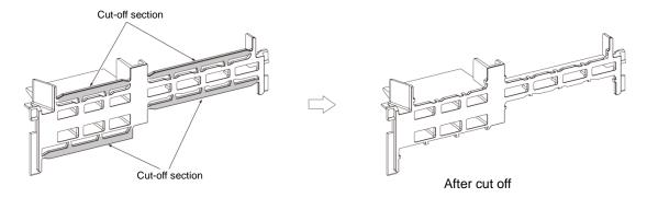
Figure 2.2-8 Wiring Guide (FRN0072E2■-4□)
