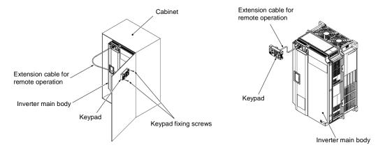
Figure 2.3-2 Attaching the Keypad on the Cabinet
