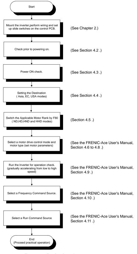
Figure 4.1-1 Test Run Procedure
