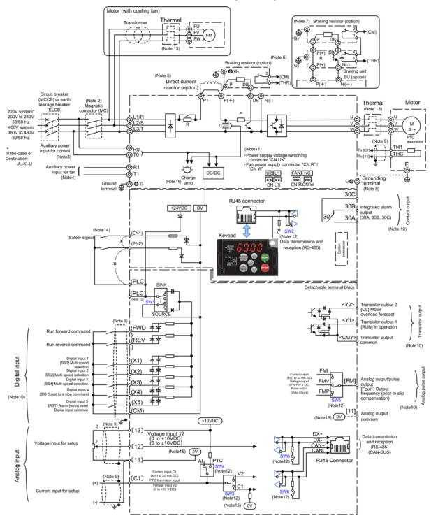
Figure 2.2-1 Standard Terminal Block Board (with CAN)
