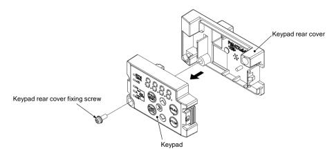
Figure 2.3-5 Attachment of the Keypad
