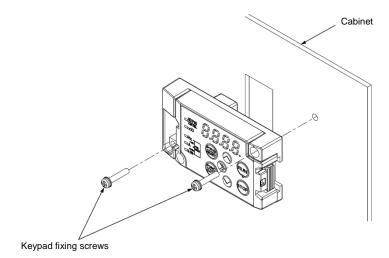
Figure 2.3-7 Attachment of the Keypad
