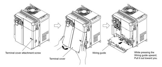
Figure 2.2-4 Removal of the Terminal Cover and the Wiring Guide (for FRN0069E2■-2□)
