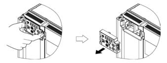
Figure 2.3-4 Removal of the Keypad
