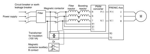
Figure 2.2-11 Example of connection of R0, T0 terminals in combination with PWM converter
