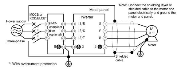
Figure G-1 Mounting an EMC-compliant Filter (option) in a Metal Panel
