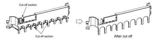
Figure 2.2-7 Wiring Guide (FRN0069E2■-2□)
