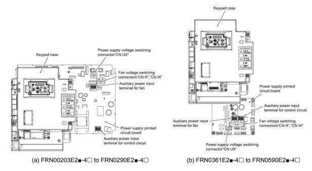
Figure 2.2-23 Switching Connector Positions
