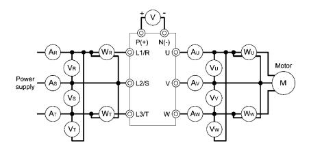
Figure 7.5-1 Connection of Meters
