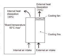
Figure 2.1-2 Installation with External Cooling
