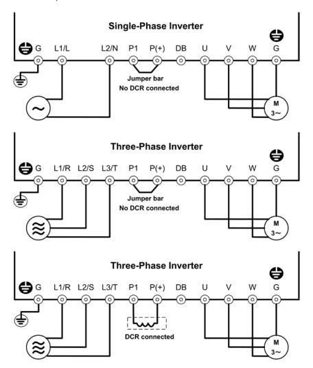
Figure 4.2-1 Connection of Main Circuit Terminals
