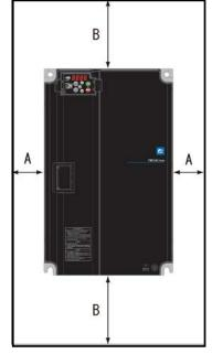
Figure 2.1-1 Installation Direction
