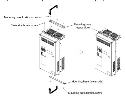
Figure 2.1-3 Method to Change the Mounting Base Positions
