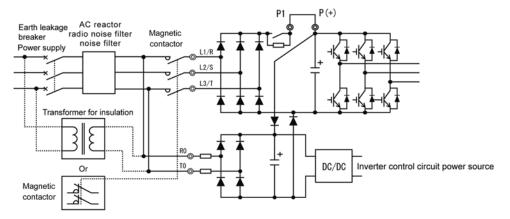
Figure 2.2-10 Connection of the Earth Leakage Breaker
