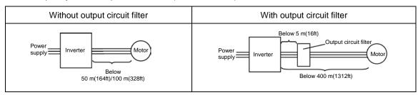
When the output circuit filter is used, the total wiring length should be below 400 m (1312ft) in case of using V/f control.
