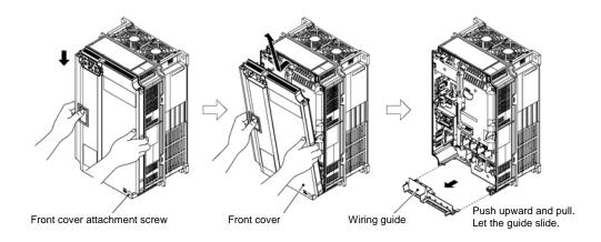
Figure 2.2-5 Removal of the Front Cover and the Wiring Guide (for FRN0072E2■-4□)
