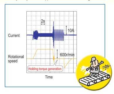
Inclusion of a brake control signal makes it even more convenient. The brake is released and applied with the right conditions at the right moment.
