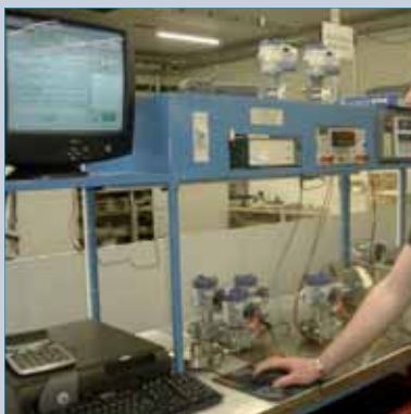
Calibration Benches : All Fuji Electric transmitters are calibrated on computer based automatic benches. The modern design of these high accurate benches ensure that even the slightest error is detected.
