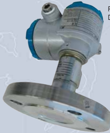
Gauge pressure transmitter with 1" - 150lbs diaphragm seal - all wetted parts in Tantalum (for high corrosive process)
