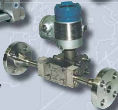
Tri Phase measurement (oil, gas and water) with DP transmitter (static pressure up to 1035 bar) on a venturi and static pressure correction via GP transmitter. (PhaseWatcher Vx developed by Framo Engineering AS & Schlumberger).
