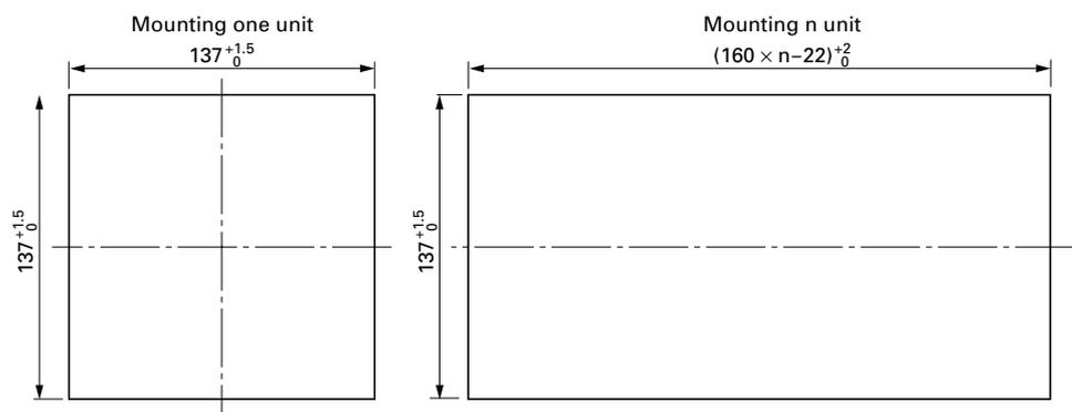
Do not use the water proof packing in case of mounting n unit
