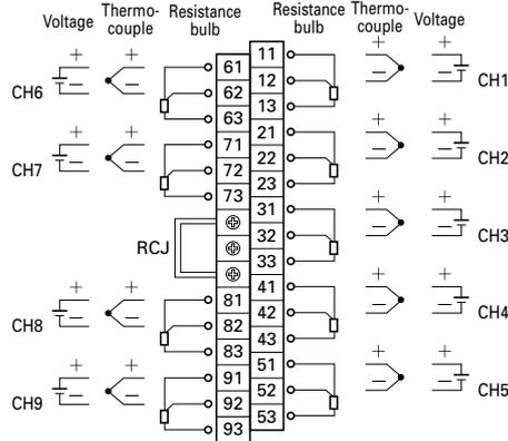
(Note) For current input, connect an optional shunt resistance to a voltage input terminal
